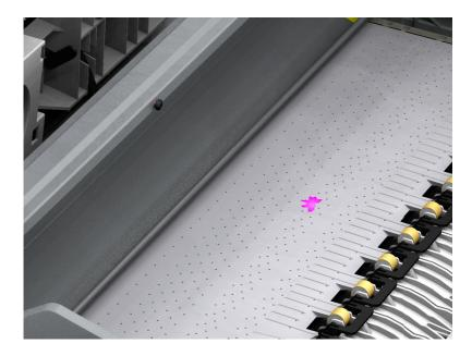
**4.** Remove the toner with the clean card. Remove the pollution from the print surface by moving the card into the direction of the toner cartridges.
